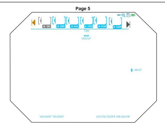
In page 5 the status bar is located in the upper portion of the screen, displays information about the actual operation state of the sight, from left to right in turn as follows:
