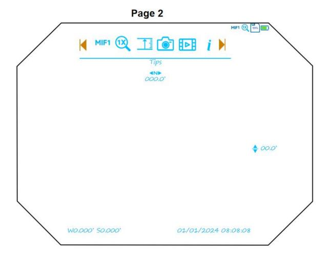
In page 2 the status bar is located in the upper portion of the screen, displays information about the actual operation state of the sight, from left to right in turn as follows:
