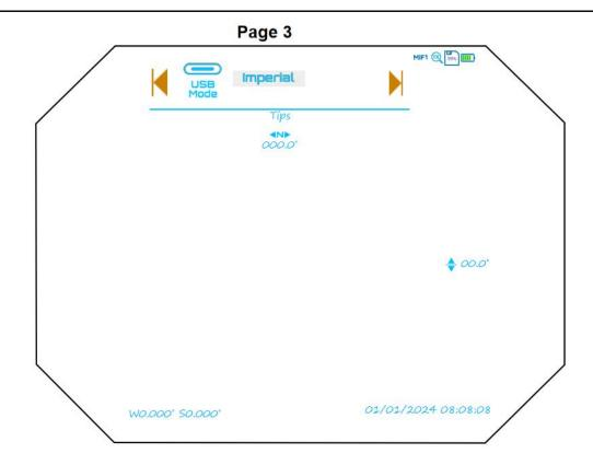
In page 3 the status bar is located in the upper portion of the screen, displays information about the actual operation state of the sight, from left to right in turn as follows:
